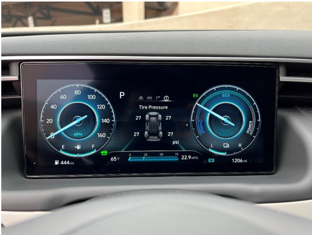
Figure 15: 2023 Hyundai Tucson display at 75 percent of placard pressure. Image Source: AAA.
