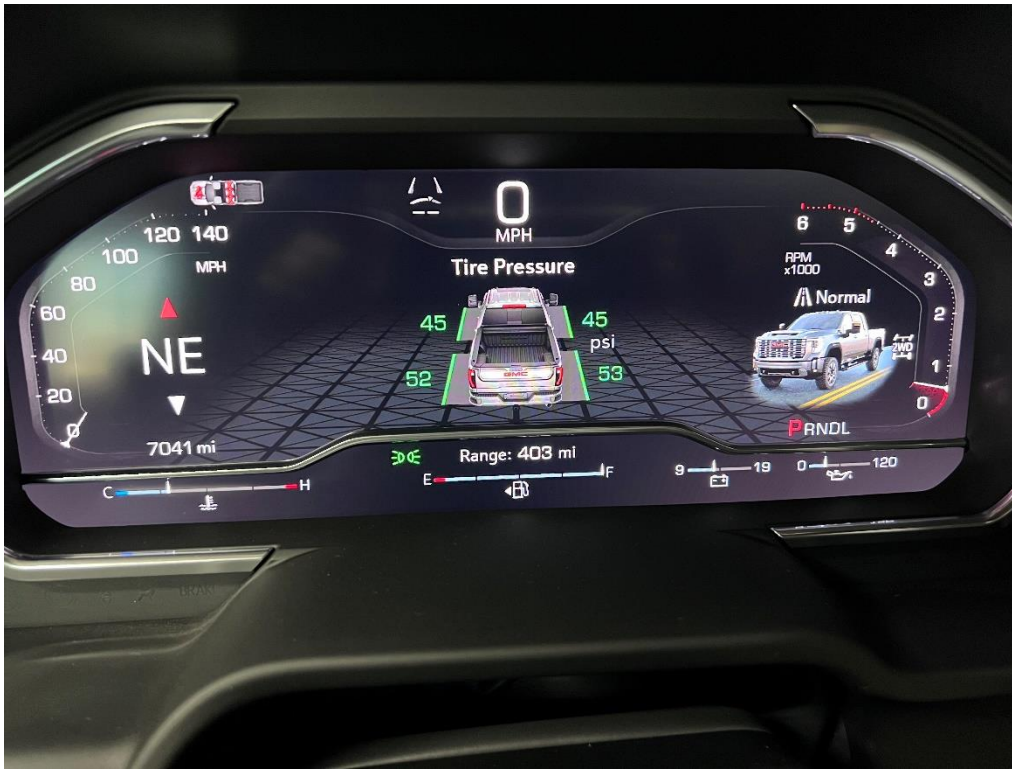
Figure 14: 2024 GMC Sierra 2500 display at 75 percent of placard pressure. Image Source: AAA.
